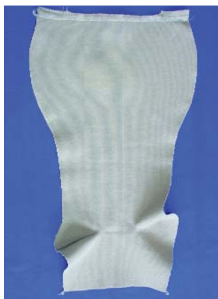
FIGURE 3 Flat knit knee high blank (before sewing) Shaped by adding and removing needles during knitting.
